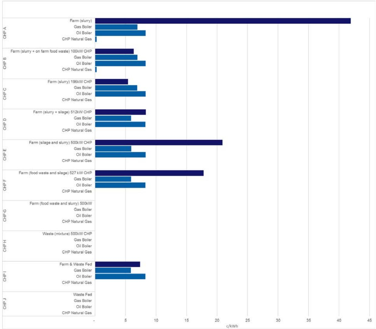
**Figure 4.6 LCOE of heat from biogas CHP: electricity valued at wholesale electricity prices**
