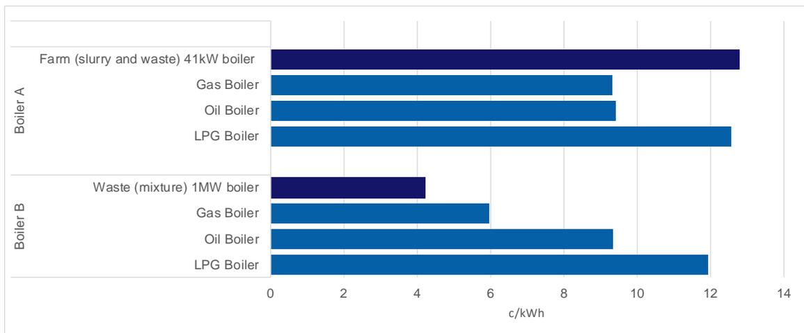
**Figure 4.3 LCOE of heat from biogas boiler: DR 12% and high heat load**
