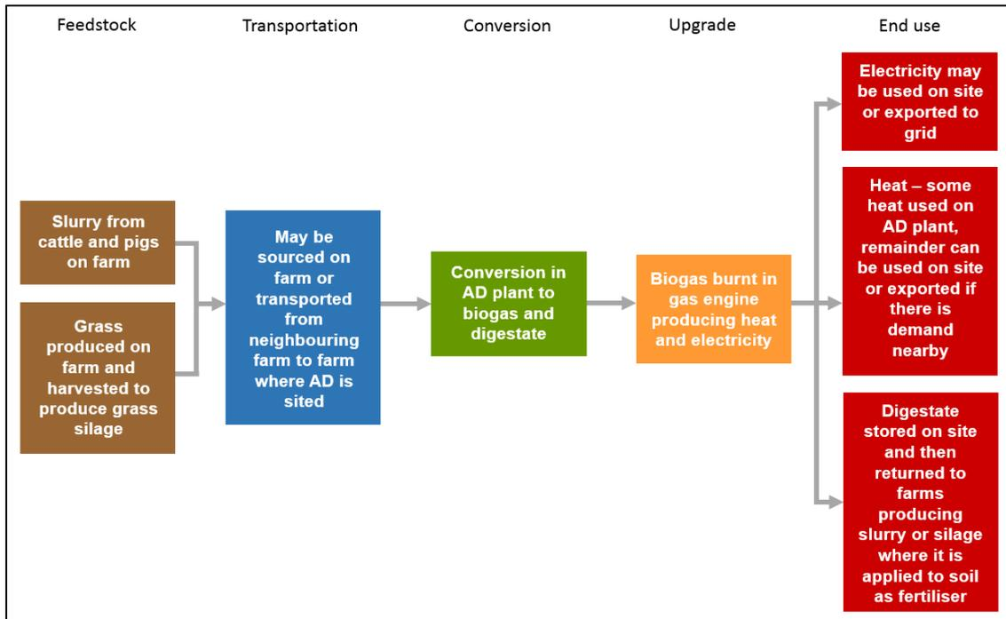
**Figure 3.11 Example supply chain for waste based biomethane plant**
