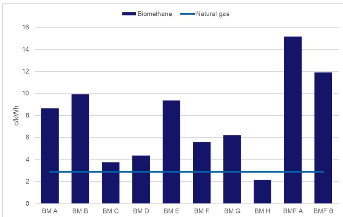
**Figure 4.8 LCOE of biomethane (12% discount rate)**
