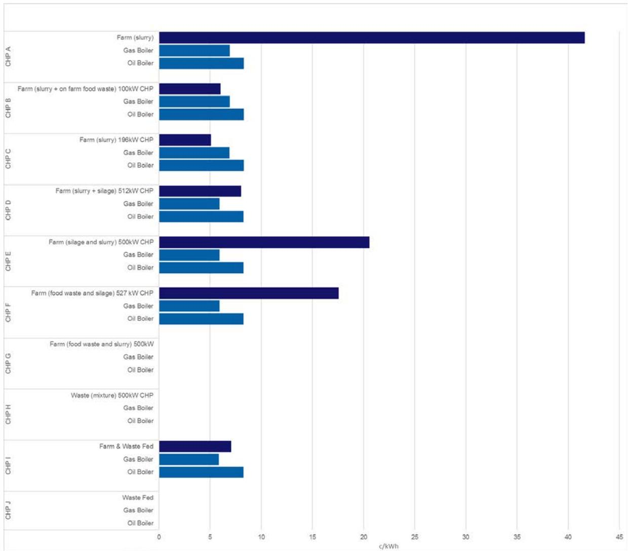
**Figure 4.5 LCOE of heat from biogas CHP: electricity valued at commercial user prices**
