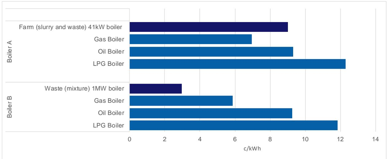
**Figure 4.2 LCOE of heat from biogas boiler: DR 8% and low heat load**
