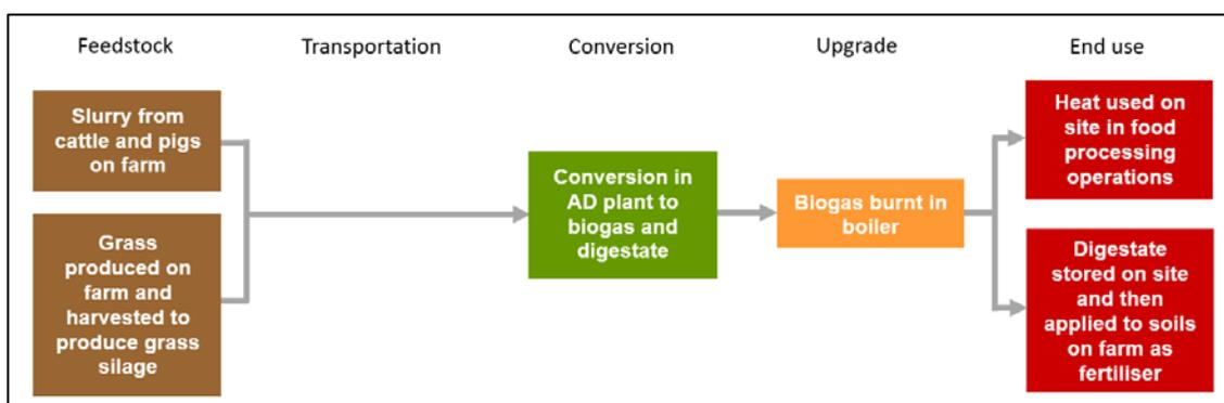
**Figure 3.10 Example supply chain for farm based AD with CHP plan**
